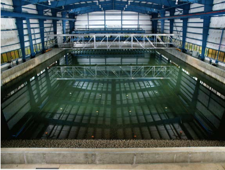
Facility: Directional Wave Basin
